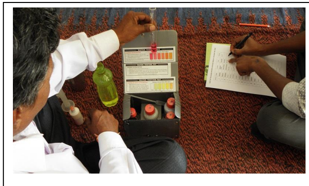
Carrying out testing for fluoride in the water
